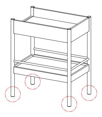
Please note stoppers on base of feet can be tightened or loosened for placement on uneven surfaces.
