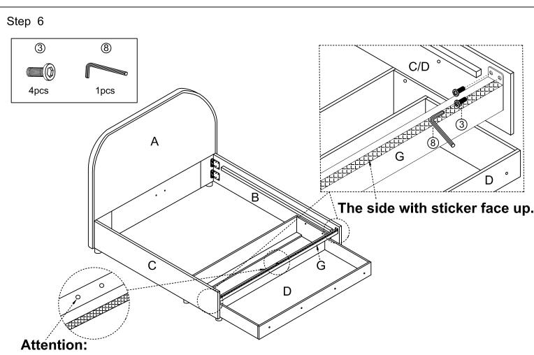
The two drilled holes on Metal Cross Bar (G) is to connect Center Rail (F). Attach Metal Cross Bar (G) to the Side Rails (B/C) with 4 x Small Bolts ③ by using Allen key ⑧. Please fully tighten all the 4 x Small Bolts ③ at this Step. Then fully tighten all the 4 x Medium Bolts ④ on the Footboard Drawer (D).
