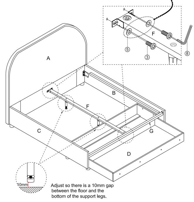
Slot the Center Rail (F) into the Headboard (A) and Metal Cross Bar (G) as shown. Secure using 4 x Small Bolts ③ and 4 x Washers ⑤, fully tightening with Allen Key ⑧ (You MUST use the Washers).
