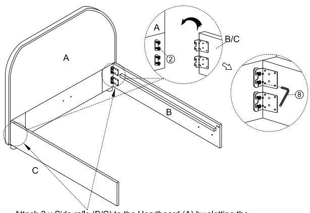
Attach 2 x Side rails (B/C) to the Headboard (A) by slotting the brackets on the Side rails (B/C) over the Big Head Bolts ② as shown. Do not fully tighten Big Head Bolts ② until Step 10.
