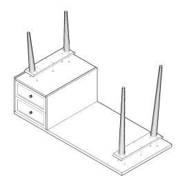
On a soft surface, such as a rug, turn the desk upside down Align the 2 legs with the pre-drilled holes
