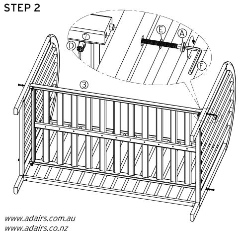
Connect the mattress base (3) in correct orientation as "This side up" indicated on frame to the two end frame with 4 connecting bolts (A)with washers (E) and 4 barrel nuts (C) at upper position.
